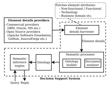
Fig. 3. Structure of proposed AERS
